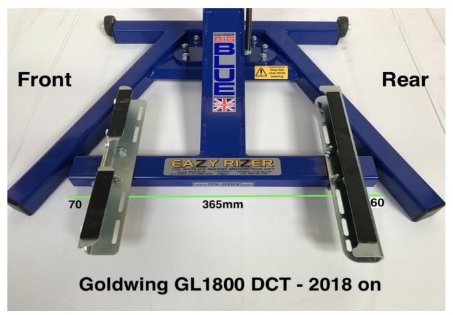
Always use ratchet type (or similar) tie down straps to secure the bike to the lift!
