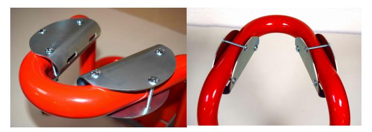
The above (left) picture shows the "Normal" position for the plates but they can also be rotated and locked off in upward positions for example the 10 and 2 o'clock if required. The Reducer plates can also be turned to an "Out of Use" position when not required (right pic)
