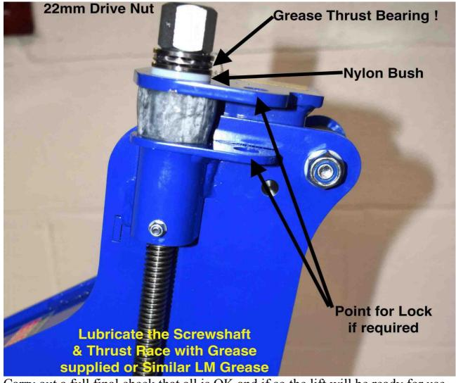
Carry out a full final check that all is OK and if so the lift will be ready for use. As the lift is raised for the first time the Large Rubber Buffer will be forced onto the White Nylon Bush at the top of the lift, avoid any grease at this point as the rubber will NOT stay in place on the nylon bush.
